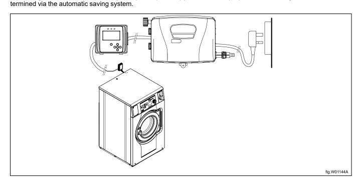
The Venturi unit operates on 115VAC / 60 Hz, 220VAC / 60Hz, or 230VAC / 50 Hz. It also supplies low voltage power to the EDS controller.
