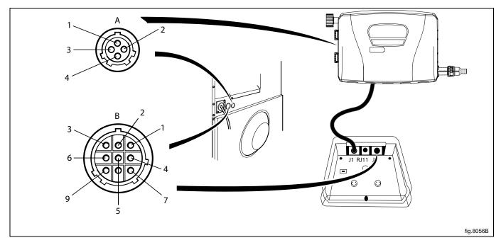
If the machine IS NOT prepared for external dosing systems from factory the cable from the J2 port on the EDS controller shall be connected to the RS232 port on one of the I/O modules in the machine. Follow the instruction for your type of machine.
