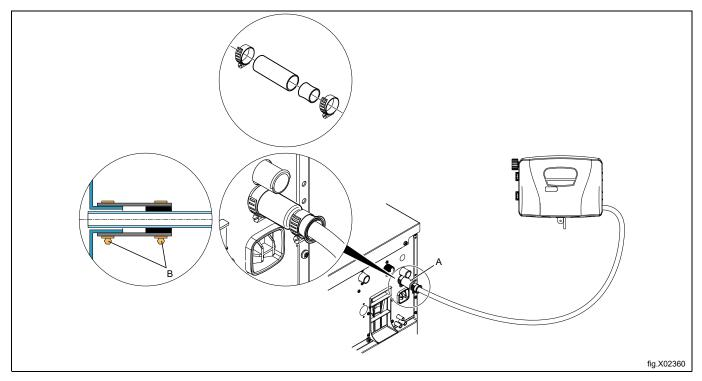
If the hoses are made of a soft material such as silicone or similar, make sure the hose size isn't reduced, isn't sharp bended and is fitted properly to the washer extractor (A). Previous figure isn't valid for the soft hose. For WH6–6 model:
