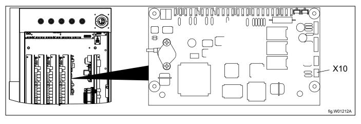
On W4400H/W4600H machines with serial number up to –980/1287 and W4850H/W41100H machines with serial number up to –1220/636, the X10 connection is NOT located at the back of the machine but in the front. In this case, the X10 connection shall not be used. Instead, it is necessary to install a DMIS kit (the art. No. for the DMIS kit is 988916197).
