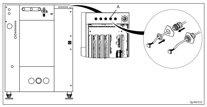
Connect the cable from the RJ11 port on the EDS controller to the X10 connection on the CPU card A1. Strap the cable at suitable positions.
