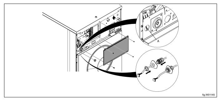
Demount the top panel and remove the cover over the connection module.
