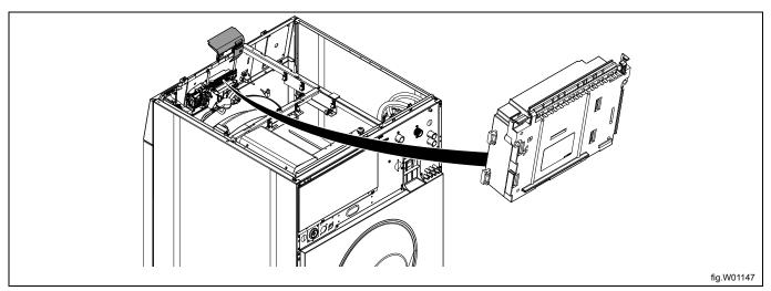
Strap the cable at suitable positions. The cable must not be in contact with the drum.
