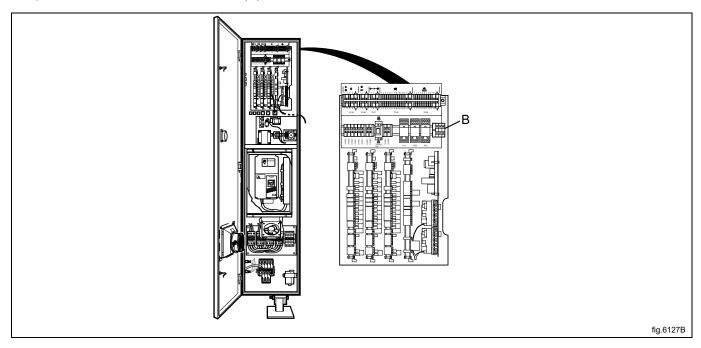
You can easily check if the machine already has DMIS installed by locating the terminal (B). If terminal (B) is connected; DMIS is installed.
