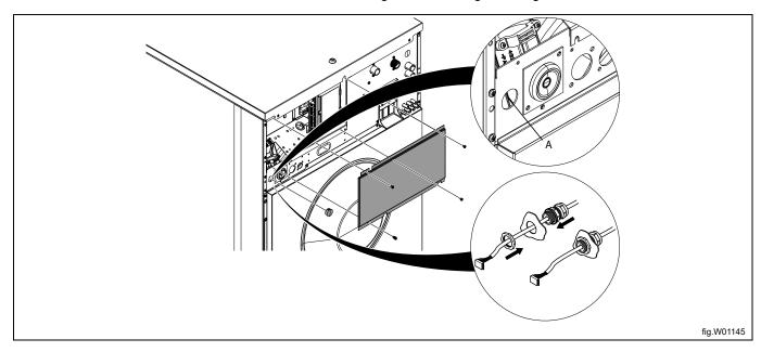
Connect the cable from the J2 port on the EDS controller to the RS232 port on the I/O module. Strap the cable at suitable positions.
