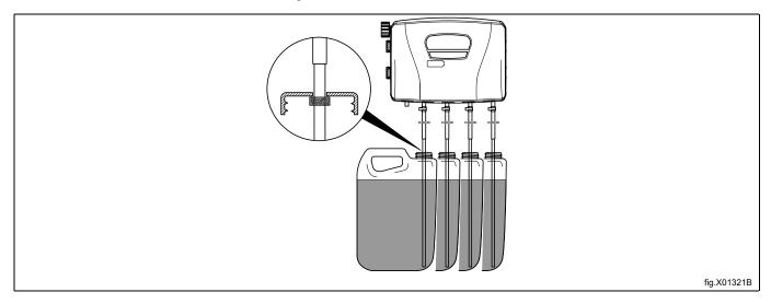
The washer extractor is prepared for connection of external dosing systems or water re-use systems etc. The connections may be closed at delivery.
